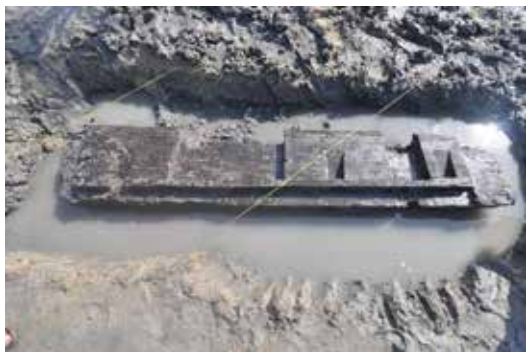
Figure 4.6 Inner surface of the hull plank; lugs show where frames or beams could be installed
